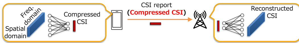
Fig. II-2.2-1: CSI compression with two-sided AI/ML model
