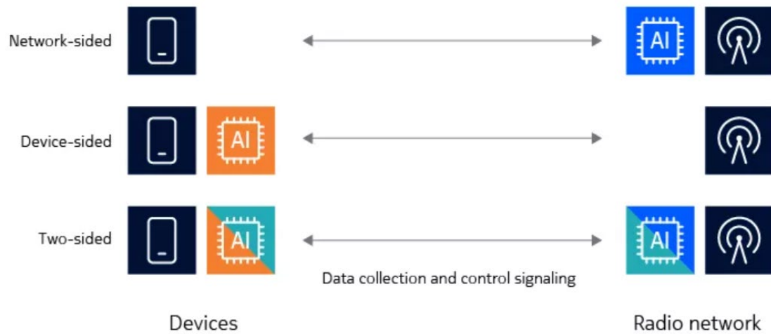
Fig. II-1.2-1: One-sided and two-sided AI/ML solutions in the mobile network air interface [3]
