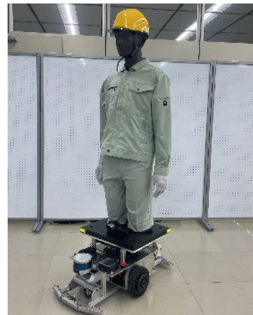
Fig. II-13.3-3. Robot-B for blocking runs between Robot-A and the 5G base station.
