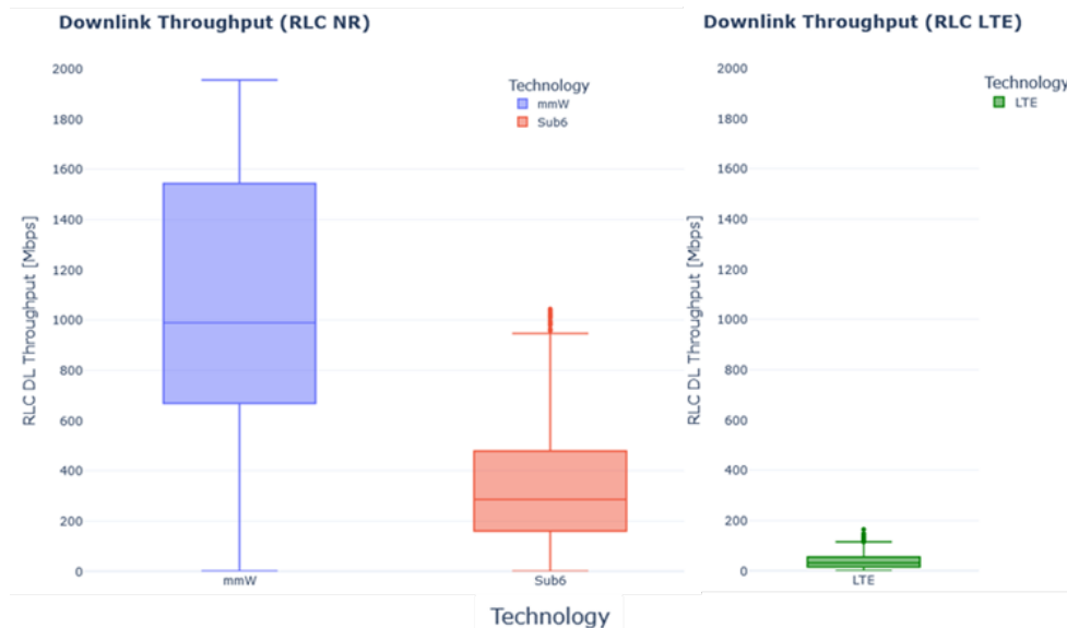
Fig. 5-8 Outdoor walking measurement of 5G mm-wave downlink throughput
