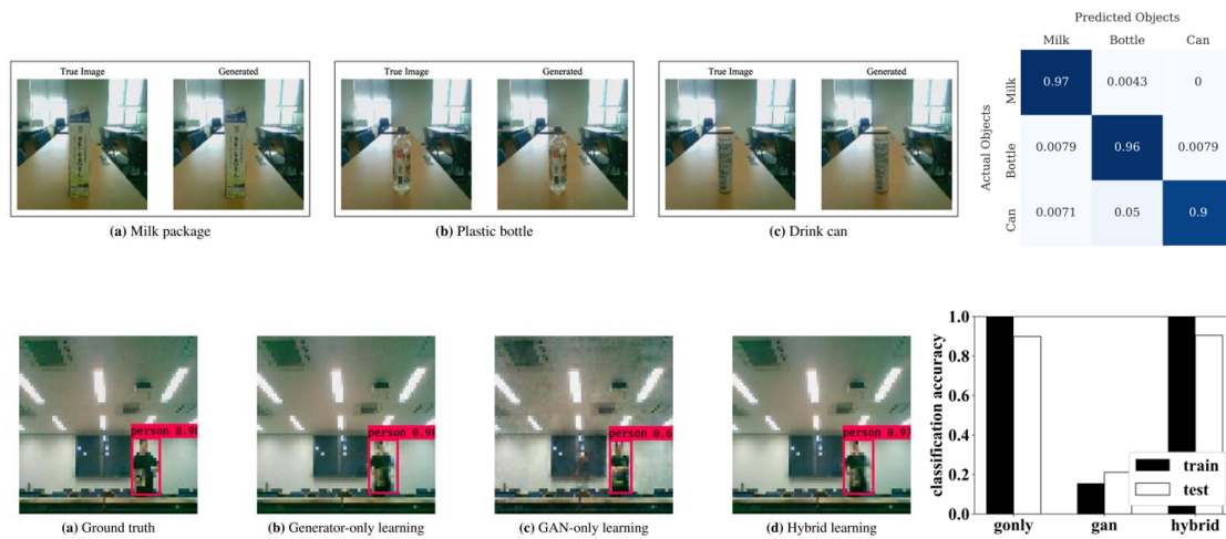
Fig. III-3. Qualitative and quantitative evaluation for different sensing tasks. (top) Object classification, (bottom) Human location classification.
