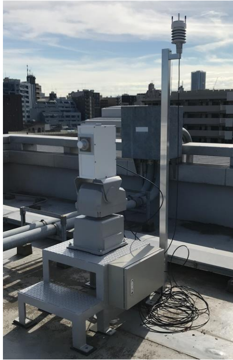
Fig. XIV-5. Outdoor radio unit mounted on a motor-controlled platform.
