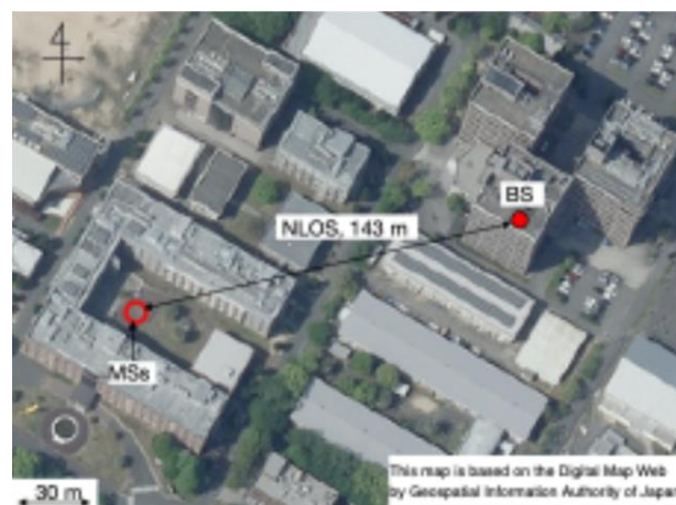
Fig. II-3-2 Measurement campaign field and layout.
