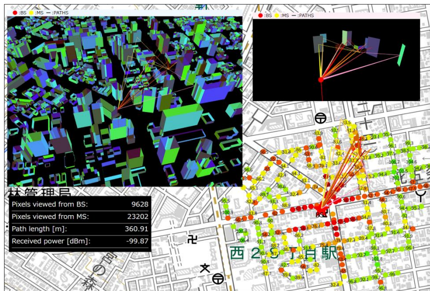
Fig. II-29. The area evaluating tool using the CIM
