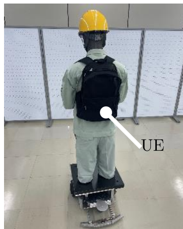
Fig. II-13.3-2. Robot-A with UE communicates through the 5G base station.
