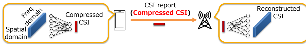
Fig. II-2.2-1: CSI compression with two-sided AI/ML model
